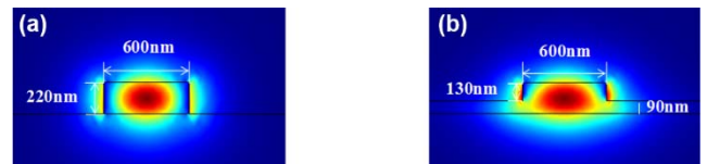
Fig. 4. The calculated TE mode optical field distribution of the (a) strip waveguide and (b) rib waveguide with 130 nm etching depth.
